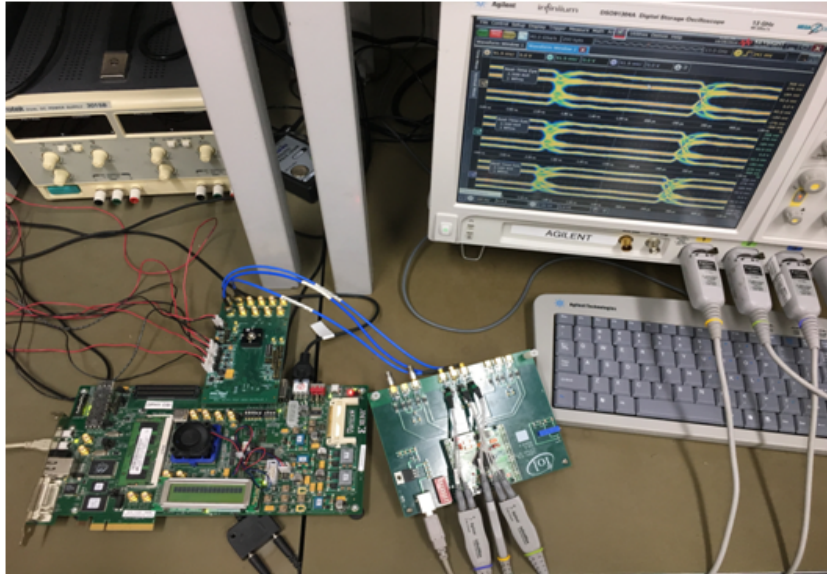
MIPI C-PHY Transmitter Testing Set-up
