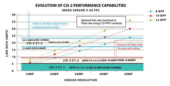
The following figure illustrates the benefits of CSI-2 logical port configurations with embedded clock and data. A myriad of imaging use cases can be mapped on multiple port configurations. Embedded clock and data (CD) lanes provide configurable logical port realizations on CSI-2 platforms.
